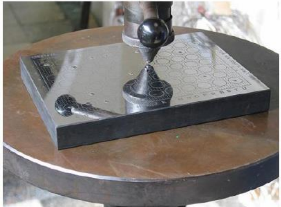
Brinell hardness testing: Calibration block
