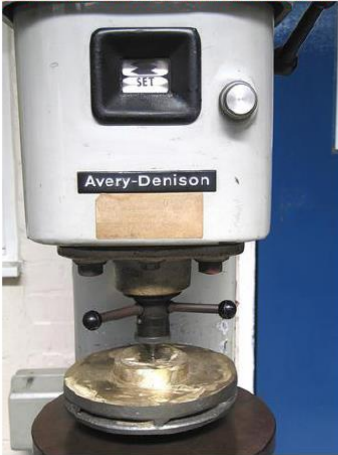
Brinell hardness test: Set position
