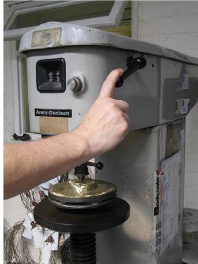
Brinell hardness test: Applying load
