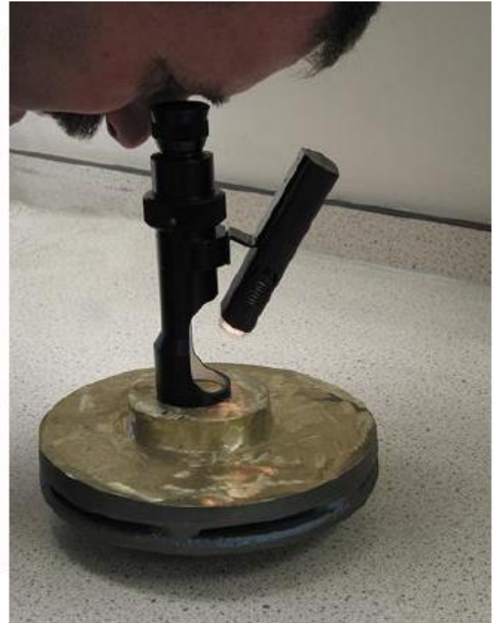
Brinell hardness test: Reading ball impression
