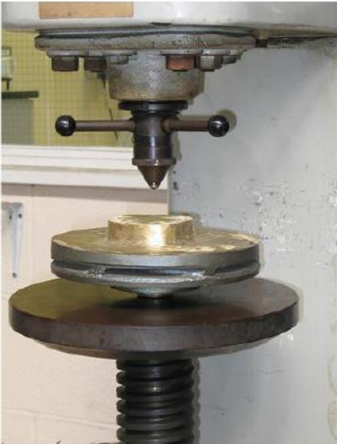
Brinell hardness test: Ready for the test
