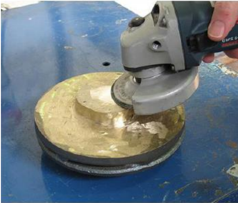
Brinell hardness testing: Surface preparation
